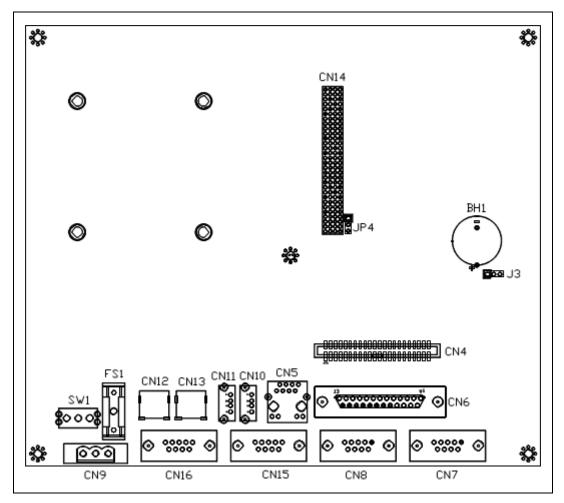
Figure 3-1. Main Board Jumpers and Connectors
